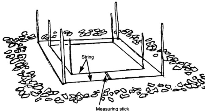
Figure 1: Marking out for a square building
